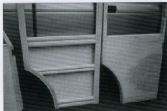
RIGHT -- Outside and inside views of newly constructed rear doors.
