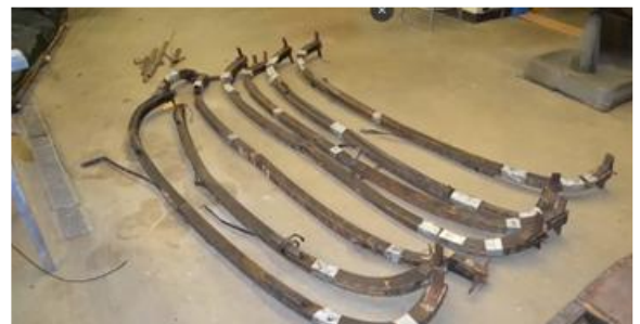
Original wood roof bows marked for duplication
