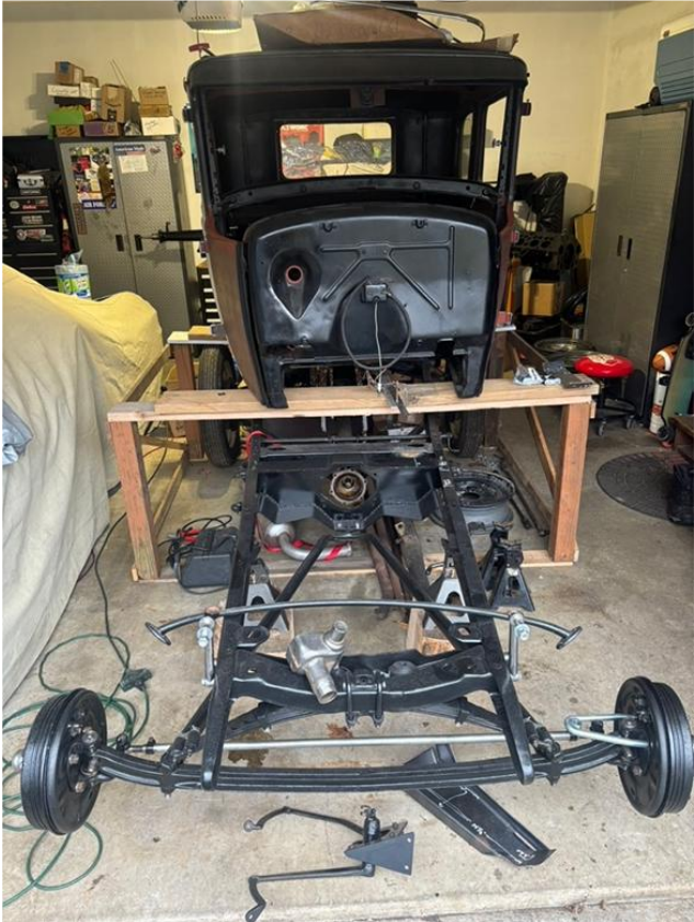
Front chassis section with complete front suspension and engine mountings
