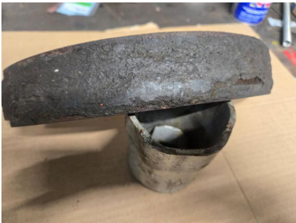
Brake shoes turned into mush from leaky wheel cylinders
