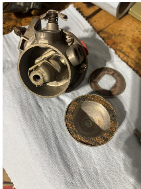
The handmade gasket fits across the top lip of the pump completely
