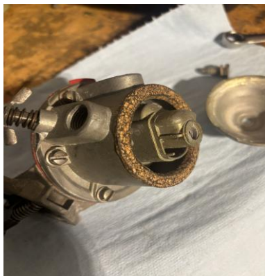
An undersized kit gasket in the pump lid
