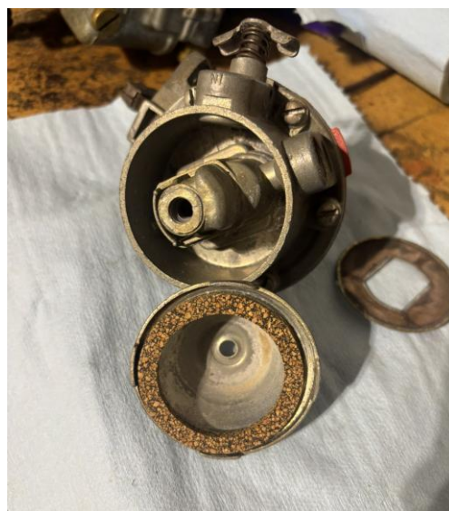
A handmade cork gasket fitting nicely in the lid
