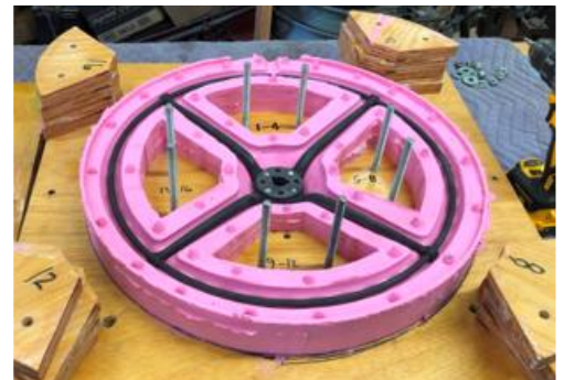
Armature inserted into the bottom half of the mold
