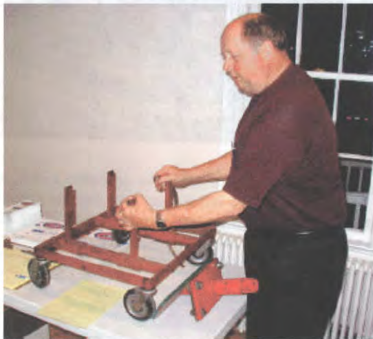
Bob Hellems shows the roll around engine stand and engine adapter for rotating stand that he made up
