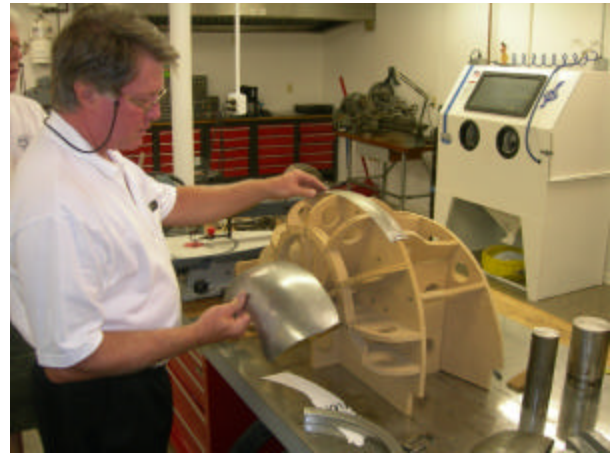
Here Steve Pieper is demonstrating a form that is used to determine the shape of a scale 1936 rear fender. The metal is shaped and compared.
