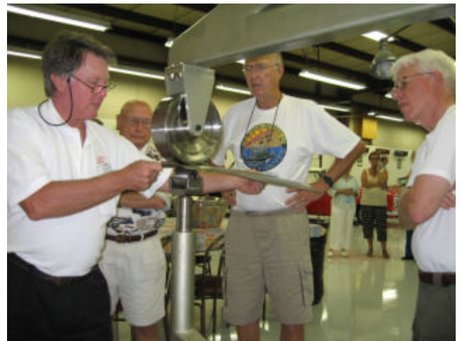
Steve demonstrated all his metal working machinery including this English wheel. He designed and made the frame to hold the wheels.
