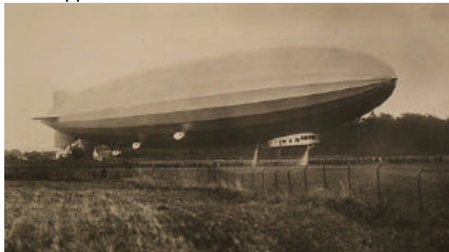
LZ-126's first test flight in Germany, August 27, 1924 – note the streams of ballast water being dumped to achieve positive buoyancy
