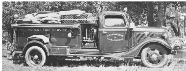
Darley-built pumper equipped to fight forest fires from Lorin Sorensen's "The Commercial Fords"
