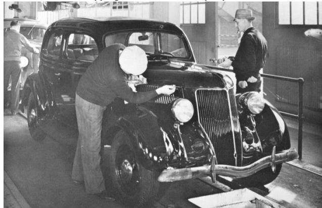
Laying down the pinstripe takes a steady hand
