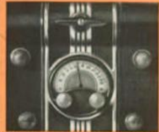
The beautiful, indirectly lighted radio dial fits into the instrument panel, in the opening ordinarily occupied by the ash tray. Matches other instruments in appearance.
