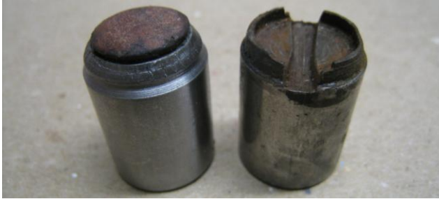
Vacuum brake plungers – guess which one is trashed
