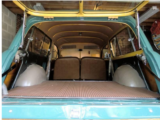
Linoleum installed – the grooves are die-straight!
