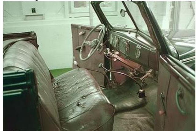
This shot clearly shows the hand controls installed in the '38 Convertible Sedan.
