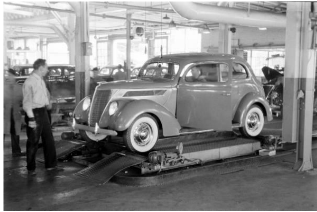
A DeLuxe Touring Sedan runs up on the dynamometer before leaving the assembly plant for a dealer's showroom.
