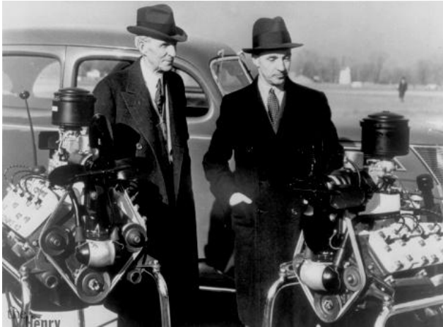
Henry and Edsel with the slightly up-dated 1937 85 horsepower engine on the left and the “new” 60 horsepower V-8 on the right.
