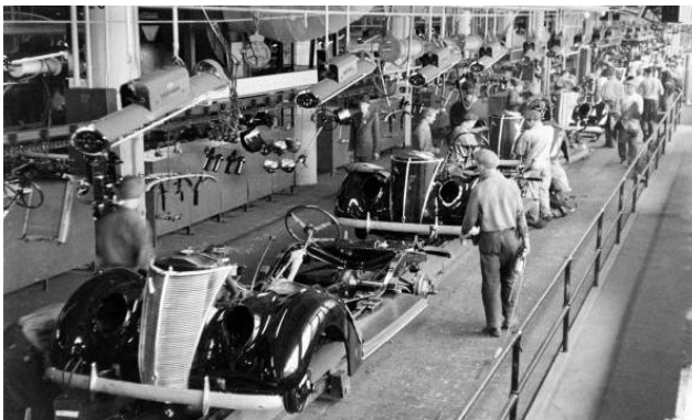
1937 Fords move down the assembly line just after the steering wheels, horns, front bumpers (in background) were installed.
