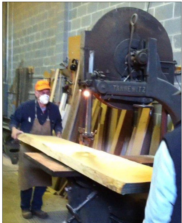
Ripping the roof longitudinal side beams at Dunlap Woodcrafts.
