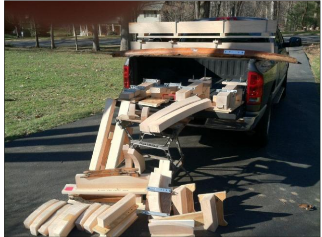
At least one finger joint is needed on each piece.
