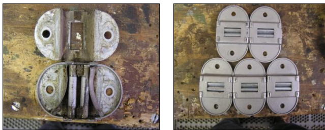
Before and after shots of the rear and middle seat retainers.
