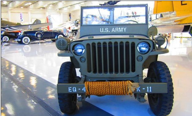
Aha, another Ford product! This Ford-built 1943 GPW or "Jeep" is powered by a 134.4 cid 4 cylinder engine delivering 54 HP.
