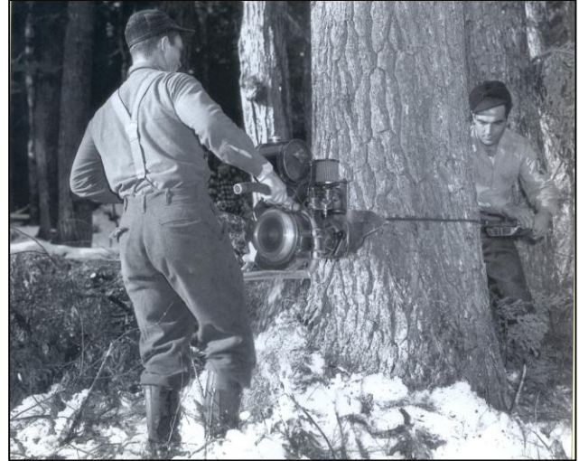
Ford lumberjacks use a two-man chain saw to harvest timber on Michigan's Upper Peninsula – no eye or ear protection here either!
