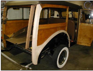
Cliff replaced the right rear D pillar and wheel surround
