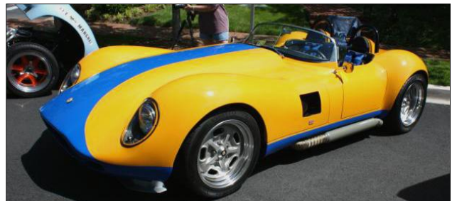
Custom built body on a ‘58 Jaguar frame with a 675 hp engine
