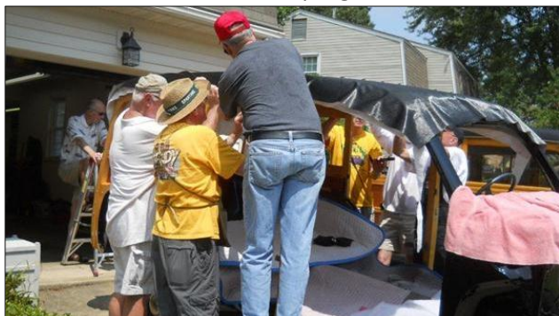
Wayne Chadderton, Dave Westrate and Keith Randall start tacking the right side after we checked to ensure the fabric grain was straight.
