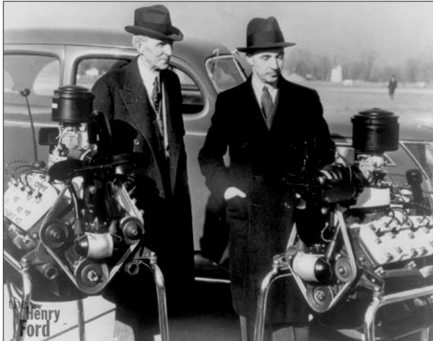
Henry and Edsel Ford at the introduction of the new 1937 Fords available with both 85 (L) and 60 (R) horsepower V-8s.
