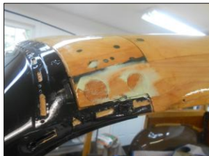
Plugging and finishing the sunken T-nut holes.
