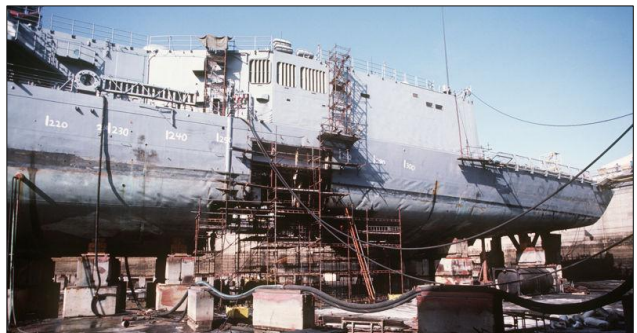
USS Roberts in dry dock after being damaged by a mine in the Persian Gulf. The 1908 mine nearly sunk the modern US Navy frigate.
