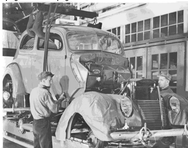
Body drop of a 1938 Standard Tudor. Notice the painted windshield frame on the Standard compared with the chromed windshield frame on the Deluxe at the top of the next column. The headlight rims hanging from the bumper guards are an interesting touch.
