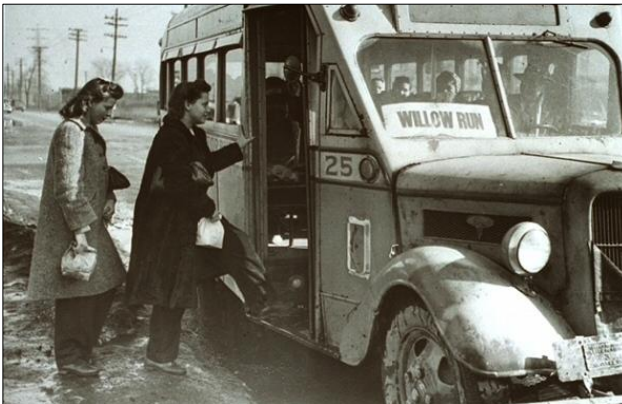
Women catching a well-worn 1935 bus to go to work at the Willow Run bomber plant. If you look closely you can see a winter front snapped in place in front of the grille shell. Brrrr.
