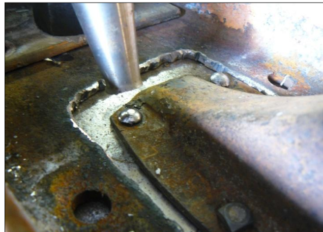
The formed rivet head and the pneumatic rivet gun.
