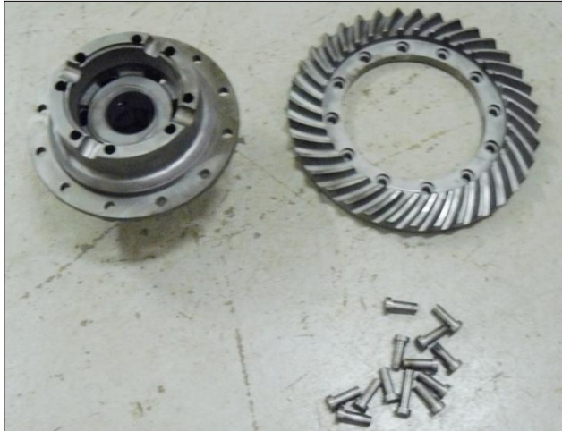
The bearing cage, ring gear and rivets ready for assembly. For proper clearance, the head of the specially machined flat head rivet has to sit in the recess inside the ring gear.
