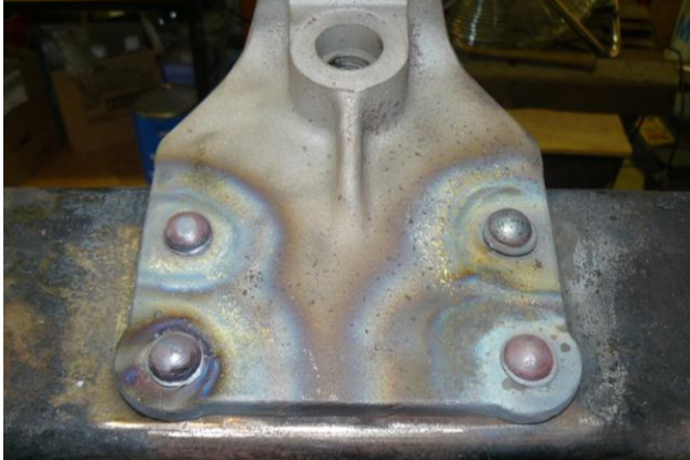
The finished product probably looks better than the original rivets.
