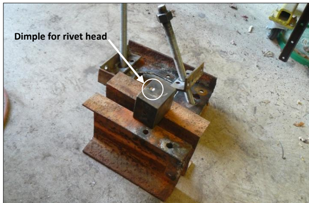
The bucking bar Dave designed and fabricated. Note to dimple cut into the backing block to accommodate the rivet head on the shaft.
