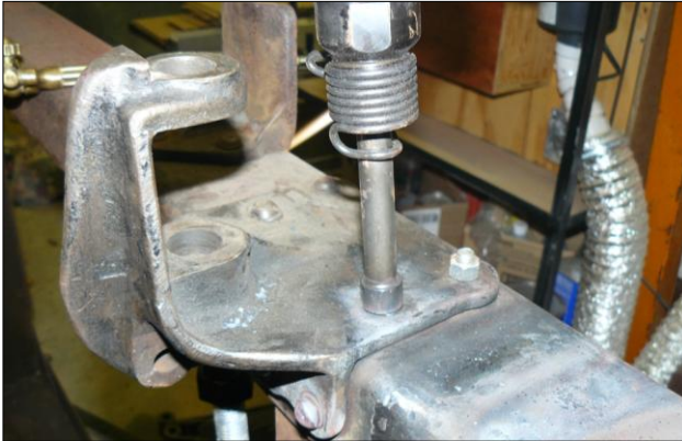
After reheating, the rivet is finished off using a pneumatic rivet gun.
