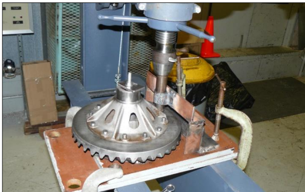
The ring gear/bearing cage assembly in the fixture as pressure is applied to the rivet shaft.
