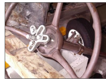
The harmonic balancer puller installed on what appears to be a 1937-39 non-banjo wheel.
