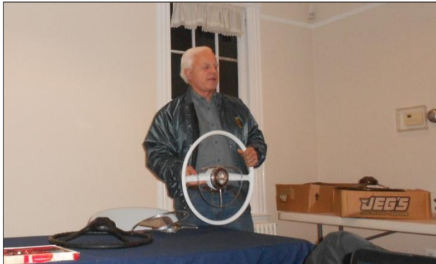
Bob and his Shoebox wheel. These wheels now had a half circle horn ring similar to the 1941 rather than the full circle 1942-6 type.
