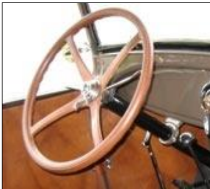
The early 1928 Model AR wheel is made of a soy-based compound that stained the driver's hands and had a peculiar smell when wet.
