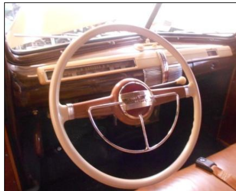
1941 was the second year that Ford used a two-tone wheel in its top models – in this case the Super DeLuxe and the first year for the horn "ring."
