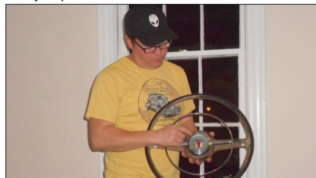
Eric's 1941 wheel with a 1946 horn ring. The gray plastic in the center of the ring matches other gray 1946 interior trim.
