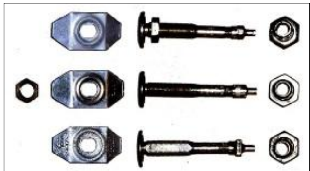
Early Schrader valves were metal and were entirely separate from the tube itself.
