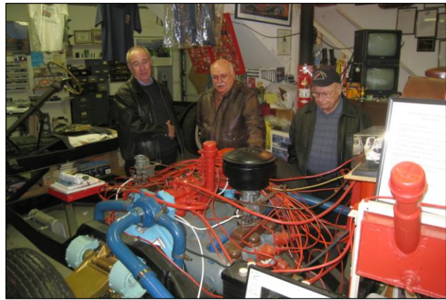
Ken Burns, Vern Parker and Hank Amster ponder the intricacies of the truly innovative prototype Tucker chassis with its mammoth engine, torque converter transmission system, independent 4 wheel suspension and 4 wheel disc brakes.
