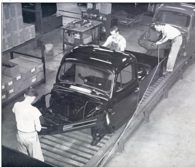
F-1s before body drop on the Atlanta assembly line, December 23, 1949, not long after “Budster” was built in Chester, PA. Check out the gas tank resting in the cab. Very interesting that at this point hood is attached upside down and it appears the rear fenders are in the bed.
