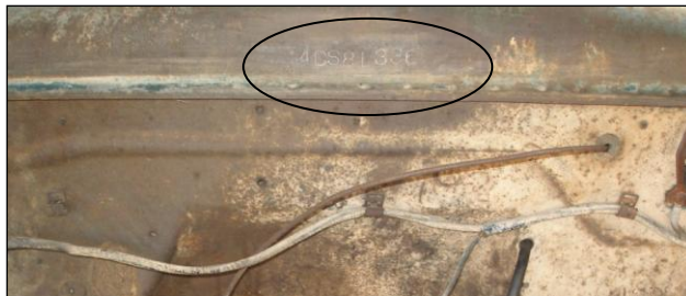
The serial number was hammered in just above the firewall seam.
