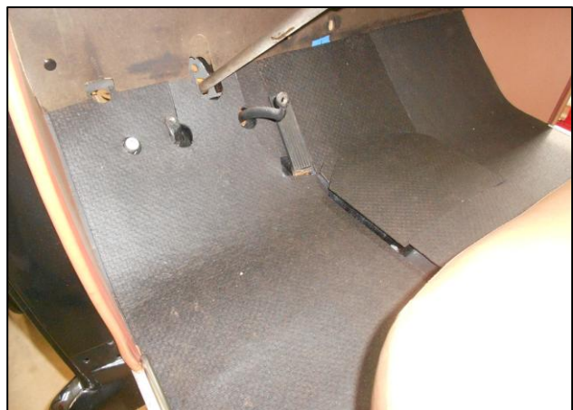
The insulation and front floorboard will need to be removed to install the engine and transmission but all cutting/fitting is now done.
