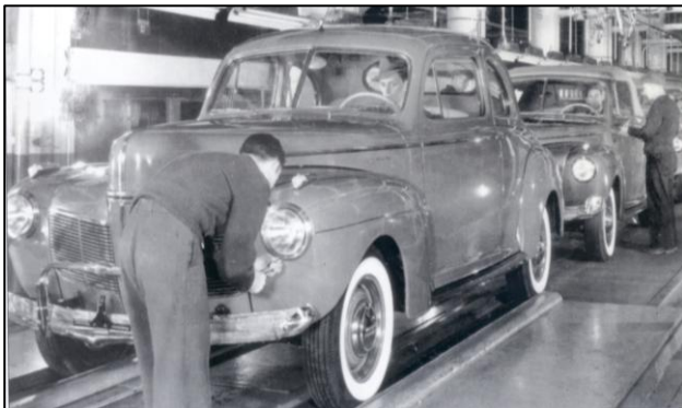
A 1941 Mercury Coupe gets a final headlight adjustment before leaving the assembly line.
