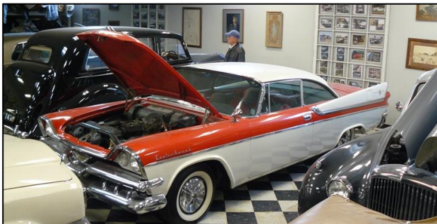
The 354 inch, dual 4 barrel Hemi in this '57 Dodge Custom Royal Dodge cranked out 340 horsepower – Dave Gunnarson photo.
