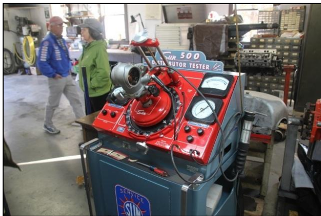
Bill had a '37-41 distributor set up on his Sun 500 diagnostic machine while we were there – John Sweet photo.
