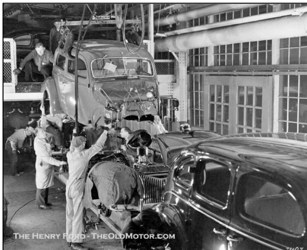
A Deluxe 1939 Ford Tudor body is lowered onto its chassis. This car might have been a special order. The page affixed to the windshield was probably the "build sheet" and it looks like the car has a radio antenna installed on the roof between the windshield wipers.
