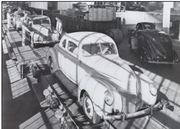
Nearing the end of the assembly line, these 1939 Deluxes have their new hydraulic brakes tested and adjusted as needed to provide smooth, quiet and safe stops.
