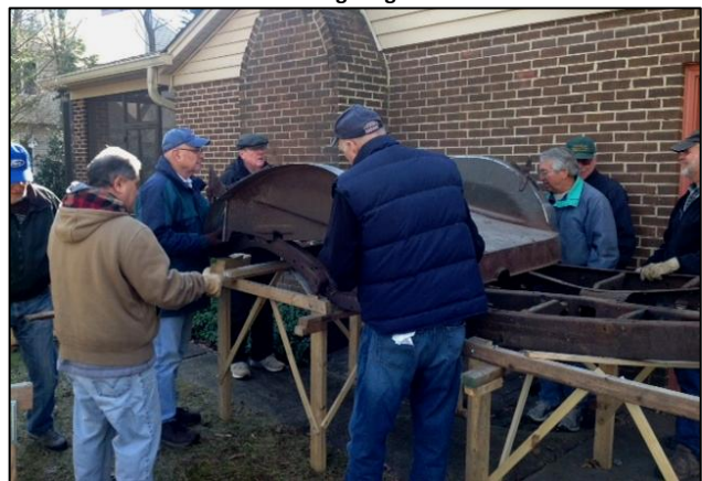
The rear floor pan is set in place on the frame.
