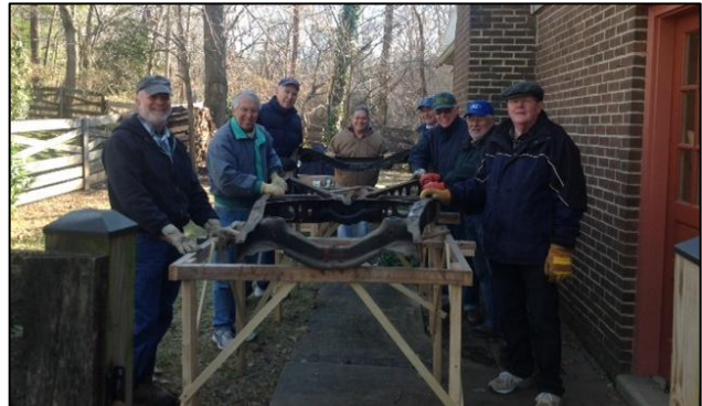
The frame sits on the working-height stand Dave constructed.
