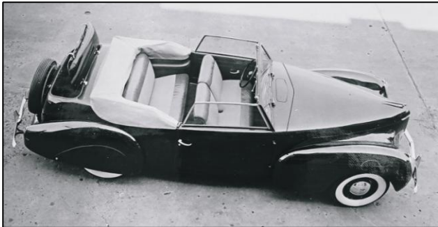
This unique shot of the second Lincoln Continental prototype show the long hood/short trunk proportions of the car. It also shows the exposed double whitewall spare tire that Edsel favored but the buying public didn't.
