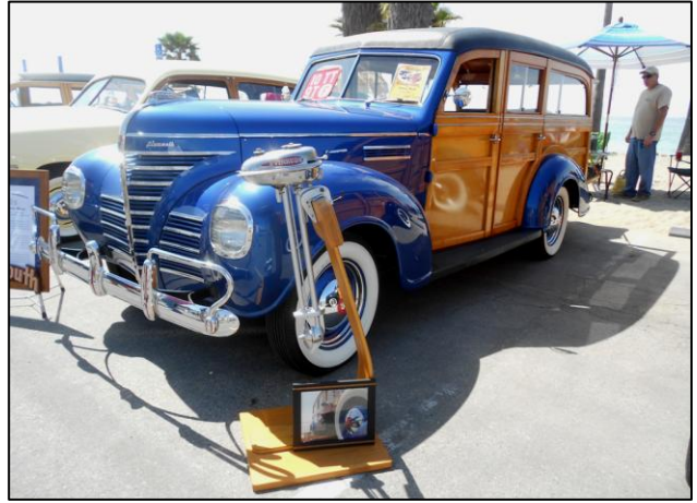
There are 2 horizontal, polished stainless steel accent strips embedded in the waistline molding on this 1939 Plymouth Woodie. I have seen contrasting wood inserts used on Mopar Woodies but never stainless before.
