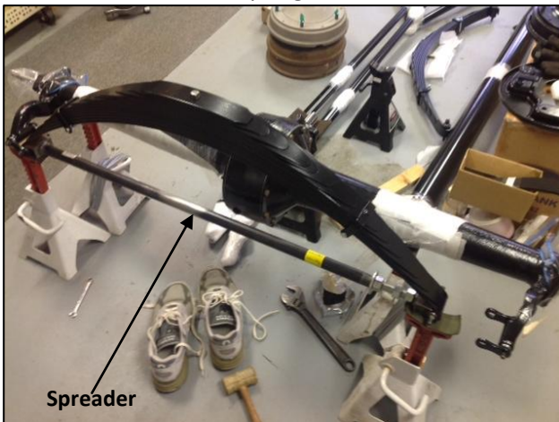
The spreader in place for re-assembly.
