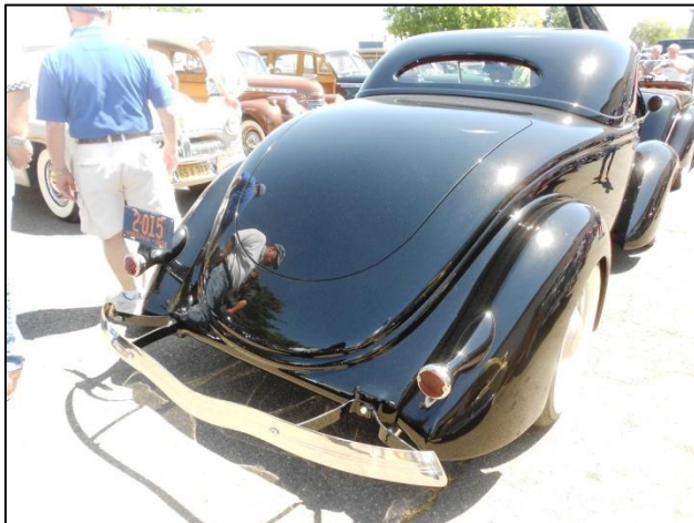
The rear deck lid opening has been modified so that its shape follows the contour of the rear body. The hard top is easily removable.
