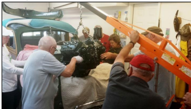
The engine begins its journey back into place.
