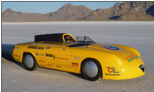
The fairing behind the roll cage is plainly visible in this picture of the record setting Alpha Spider.
