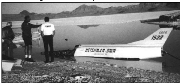
Steve's ended his last run at Bonneville in a drainage ditch when a parachute failed.
