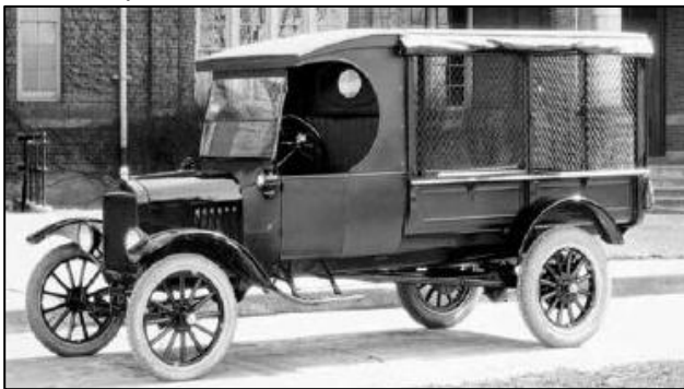
A 1924 Ford Factory Canopy Express Truck - Ford's first truck bed. This example is fitted with canopy top, screens, and side curtains.
