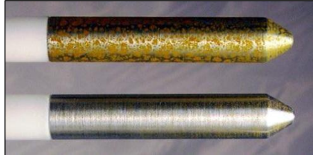
Top: a steel rod immersed in a mixture of 10% ethanol and distilled water for 24 hours at 100°. Bottom: same type of steel rod immersed in No-Rosion treated 10% ethanol gasoline and distilled water under same conditions as above.
