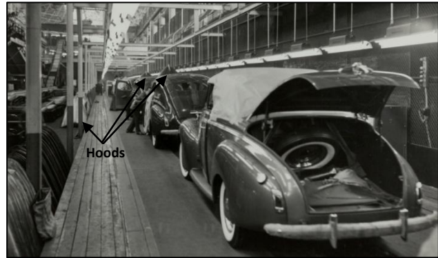
Hoods being installed on 1940 Mercurys. You can see the raised hoods on the cars in front of the Convertible. Ford and Mercury Convertible bodies were built at the Lincoln plant and then delivered to the Ford or Mercury assembly line.
