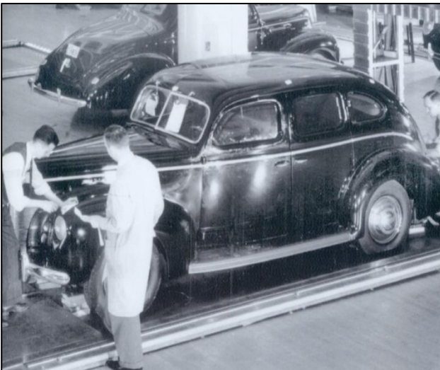
An early clay model of a 1940 Ford Deluxe Fordor in the design studio begins to show some recognizable 1940 front end styling cues: the pinched hood, sharply pointed grille with body color auxiliary side grills and sealed beam headlights.
