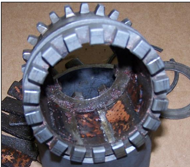
You can see the remains of the stuck cork pads.
