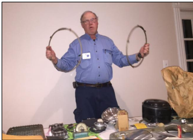
Jim Crawford displays sand filled wheel balancing devices that attached to 16" wheels and were supposed to eliminate forever the need to have your wheels machine balanced.
