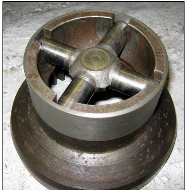
This A-24 differential case has been banded and the A-30 differential spider shortened.
