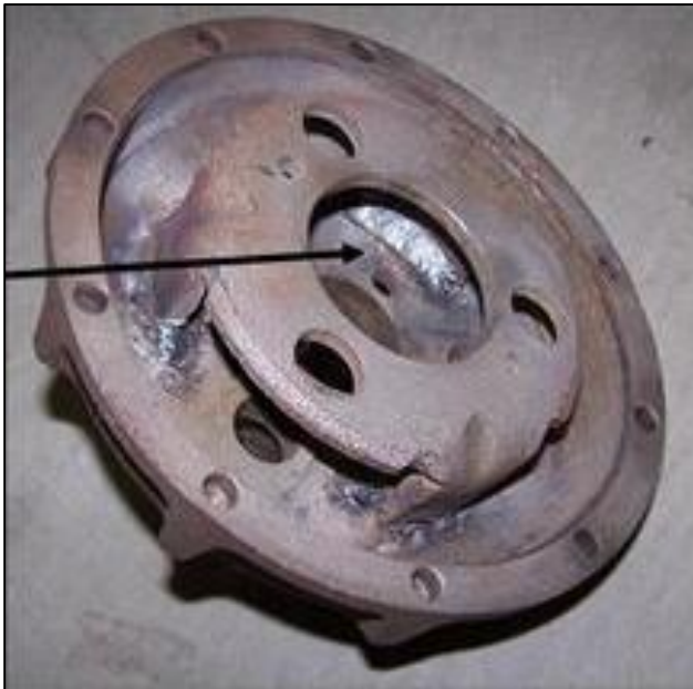
The arrow shows where the A-17 "basket" will be welded to strengthen and reinforce the unit.
