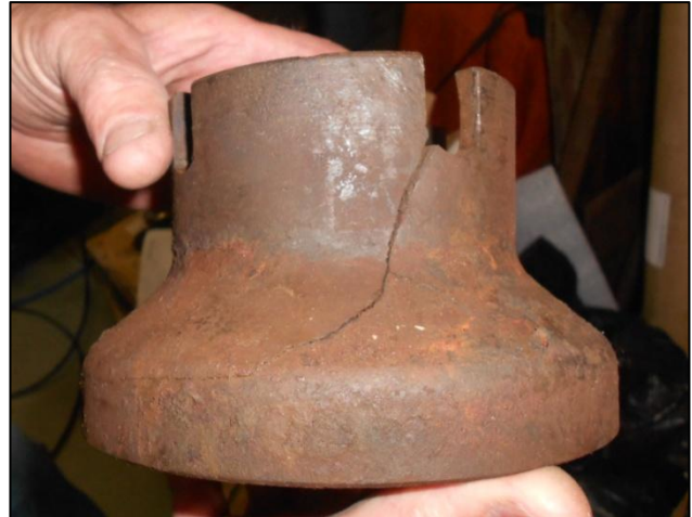
This A-24 differential case has been damaged beyond repair.
