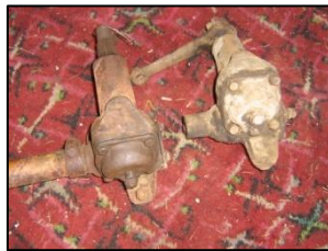
Right-hand drive steering box mounting bracket and boxes.
