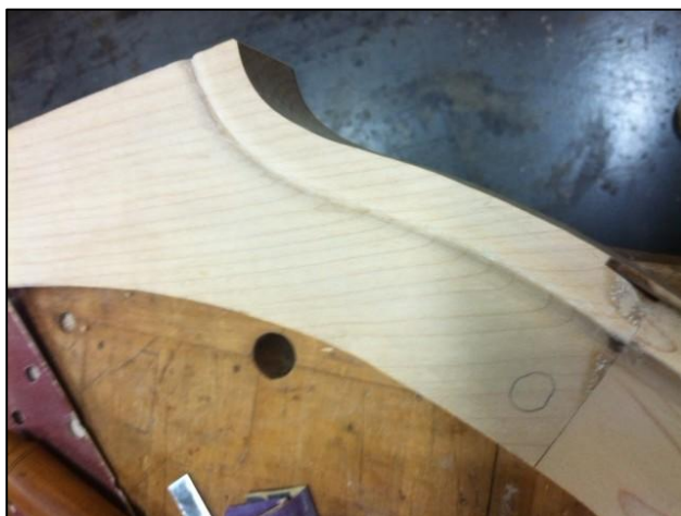
Detail of decorative bead on outside rear edge of right quarter panel wheel surround.
