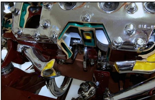
A good shot of the center exhaust port exiting through the water jacket. Again, liberal use of color. Note also the 81A-5 part number on the face of the cylinder head rather than tucked away in its usual location in the back of the head.
