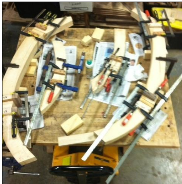
Glued up and clamped wheel surround assemblies.
