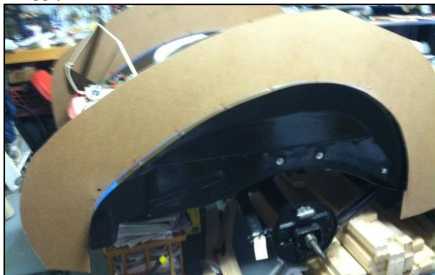
Masonite templates for the wheel surrounds.
