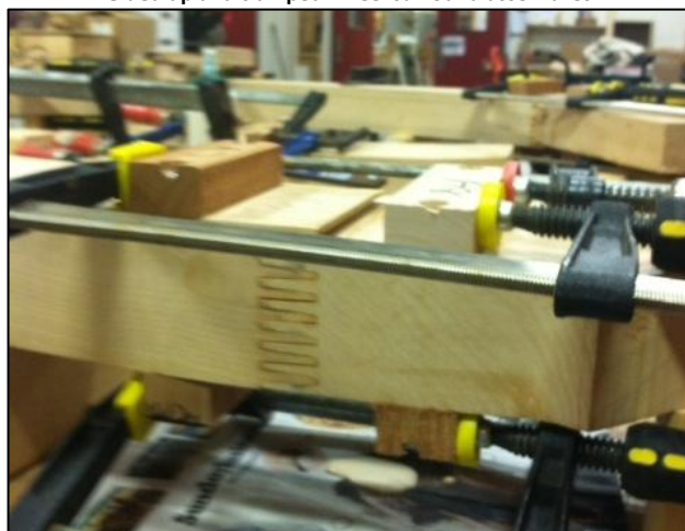
Close-up of glued-up finger joint.
