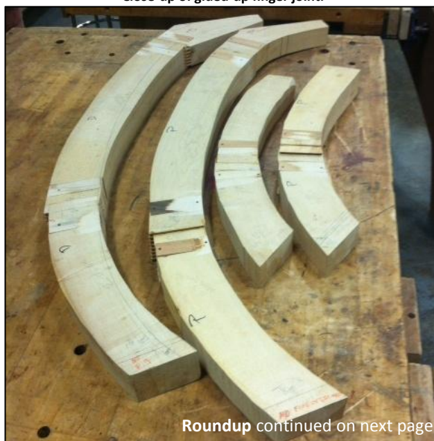
Quarter panel and rear dog legs after clamping block were removed.
