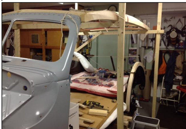
Temporary roof support structure holding the roof side beams.
