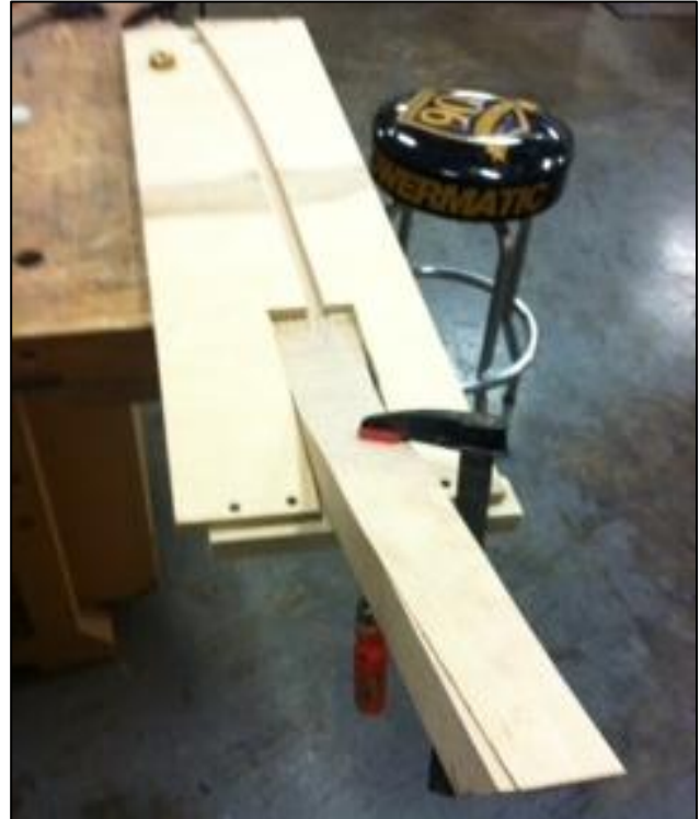
The jig set-up shows that the outside panel will be curved.
