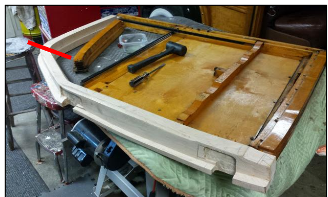
This picture shows Cliff Green in the process of replacing the front passenger door post and you can see the panel insert. The piece Dave is making ends at the red line.
