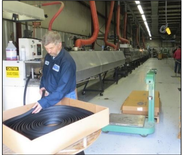
finished door seal stripping comes out the other end.
