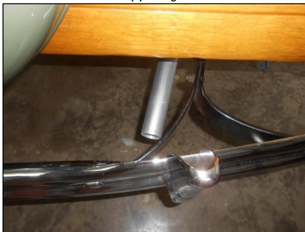
New 11A-5255-B replica installed on first Woodie.
