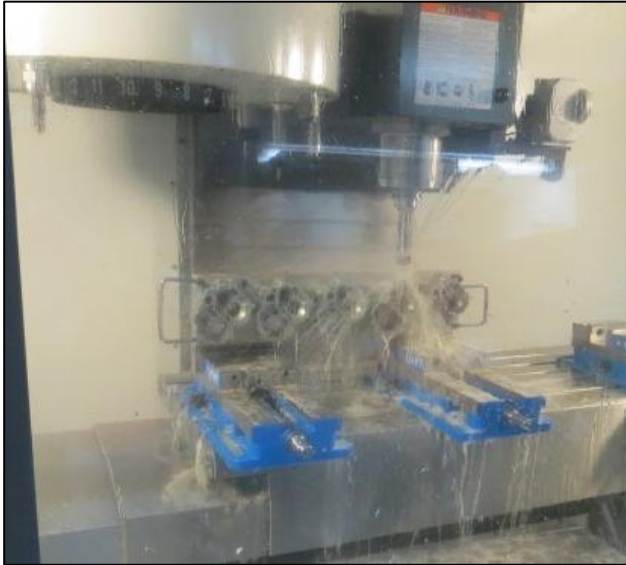
Five new Holley 94 carb bodies are simultaneously drilled by this computer-controlled machine and once assembled...
