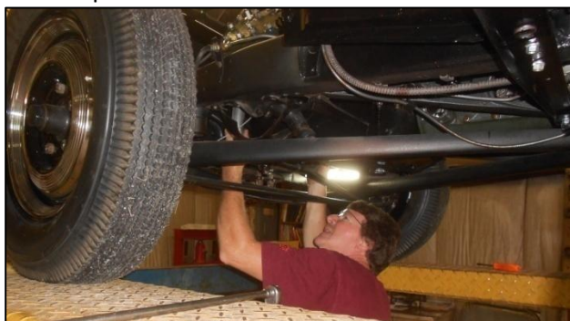
Crossover pipe being fabricated.
