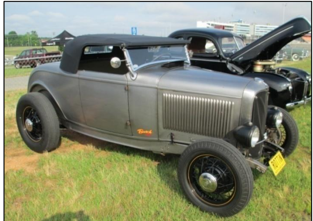
This car has a wonderful retro look: stock body, chopped windshield, wide and narrow wire wheels, '39-41 drum brakes, early shocks.
