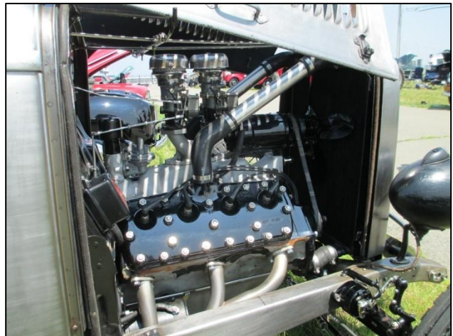
Under the hood the nostalgia look continues with a beautifully detailed motor featuring smoothed cylinder heads finished in gloss black and a vintage dual carb intake manifold.
