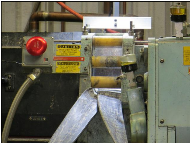
Rubber feed stock is fed into an extruder and...
