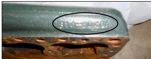
81A-6049A is a right head for a '38-42 engine.
