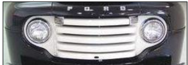
1950 F-1 grille with crank hole.
