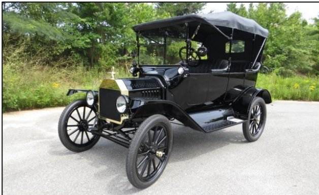
Keith's 1915 Model T is one of the last Ts to have a brass radiator shell.
