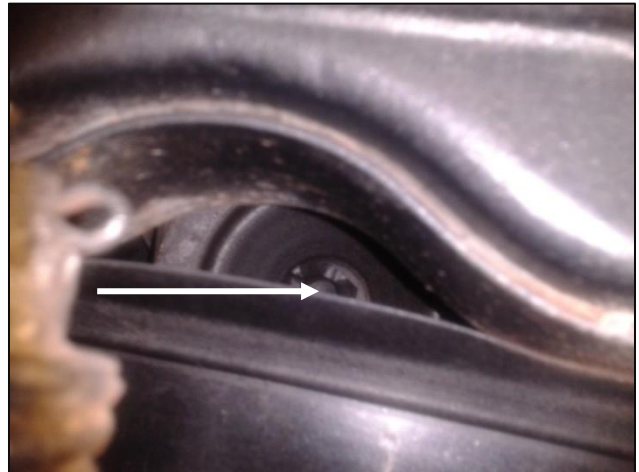
under the arch in the front crossmember before engaging the crankshaft ratchet (pulley nut) barely visible in this picture.
