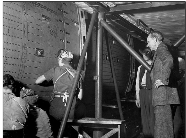
real Rosies at the Willow Run bomber plant riveting the center wing section of a B-24 as Henry Ford looks on.
