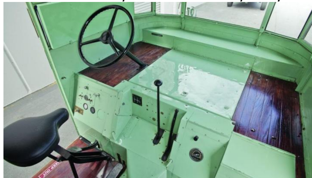
The shelf in front allowed the driver to keep his delivery tray close at hand for his frequent stops.
