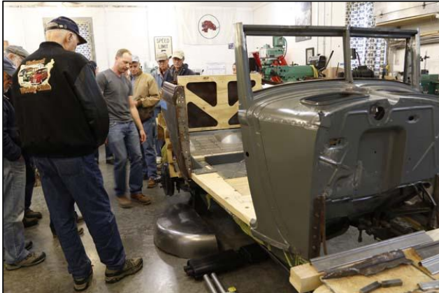
Some of the new inner wood structure is visible in this shot along with a newly fabricated rear inner fender well sitting on the floor. Check out the dual cowl vents and split windshield.
