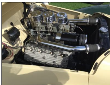
The Allard's flathead was 337 ci producing 250 bhp w/ 3-deuces
