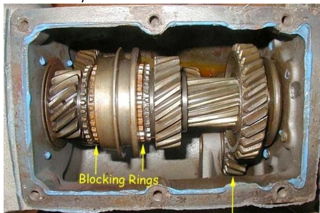
This '39 gear set has the helical cut reverse and first gears.
