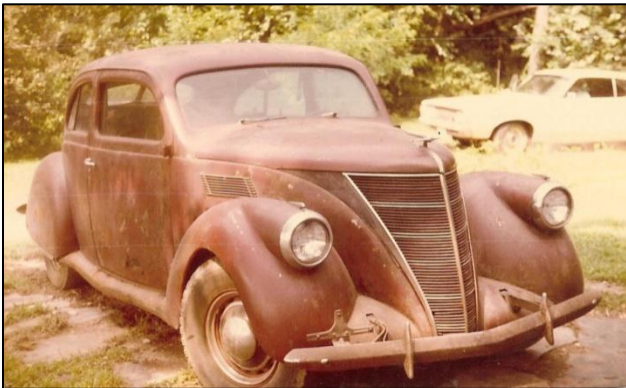
The LZ sporting sealed beam conversions.
