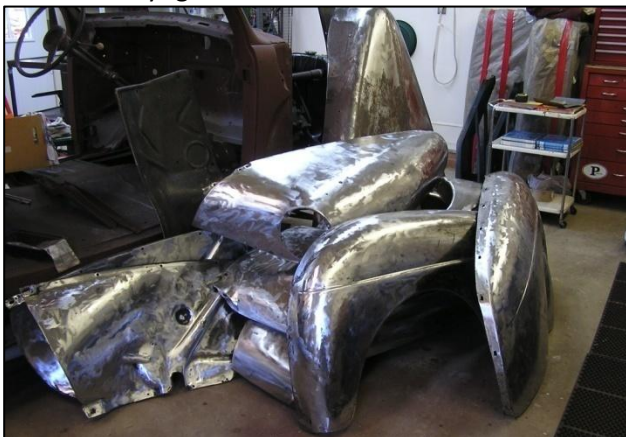
Ready for metal stripping and de-rusting.
