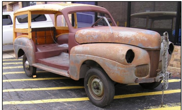
The Woodie was surface towed to the body shop. Lots of flash rust had accumulated by the time it was delivered.
