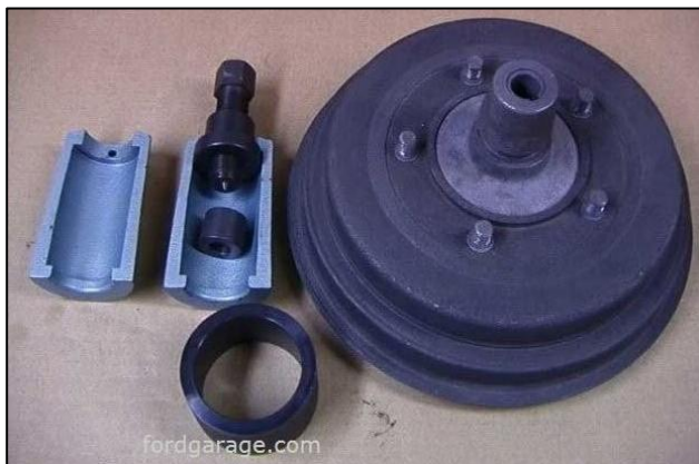
The trusty old KR Wilson ABV-156 hub puller didn't work.
