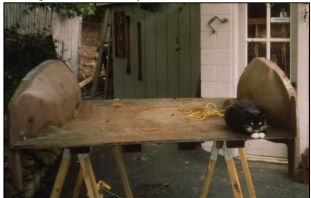
The original rear deck was usable but needed quite a bit of work. A new tool compartment had to be fabricated and the area where the wood meets the inner fender panels was rusted and needed to be replaced.
