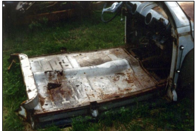
The floor original floor pan and rockers were rusted beyond repair so Bob bought this rust-free floor pan from a vendor in the mid-west.
