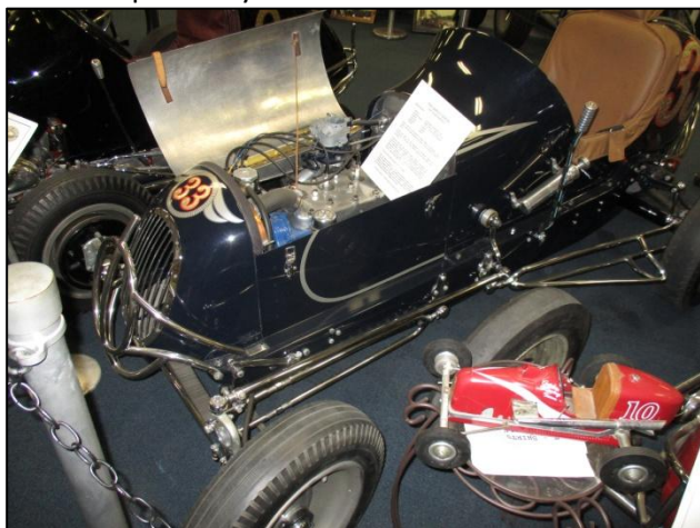
The DeRicci Fergie #33 Midget was built in 1941 (there's that year again) using a modified 119 CID N-9 Ford-Ferguson engine. These engines, when highly modified, were competitive with V-8 60s and Offenhauser-powered midgets in the 30s and 40s.
