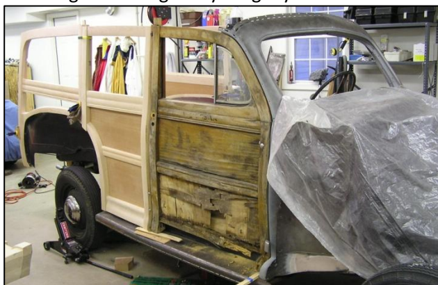
Mocking up the right side wood – Powder Post Beetle damage completely destroyed the bottom of the original front door.
