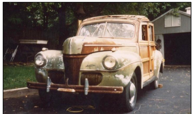
That's an original 1940/1 sealed beam headlight in the left fender.
