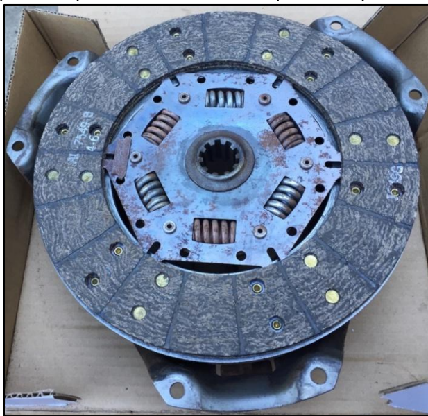
New clutch disk. New throwout bearing. Pressure plate was good.
