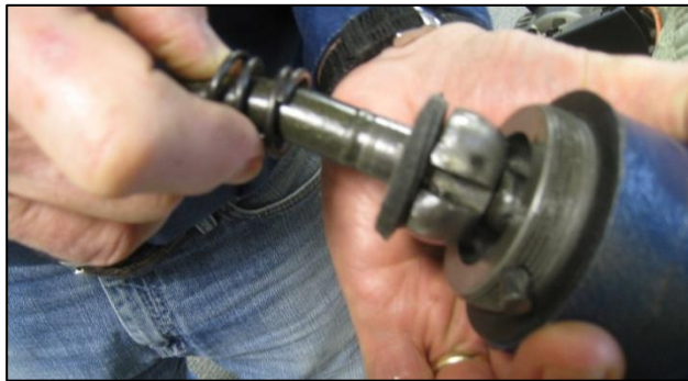
The worn shift lever fulcrum and pin.
